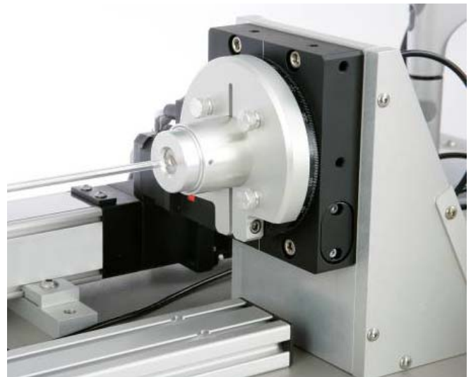
Figure 1: Rotational Stage with Removable Collet
